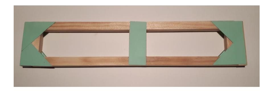
Glue the three 2 \(^3\engline^n - 60\text{mm}\) axles into the holes of a drilled 3 \(^5\engline^n - 90\text{mm}\) piece. The dowels are to flush with one side and this is covered by a 3 \(^5\engline^n\) by \(^3\engline^n\) (90mm by 10mm) cardboard strip cut from the green card. Use the other drilled 3 \(^5\enline^n - 90\text{mm}\) piece to ensure that the axles are perpendicular to both of the pieces.
