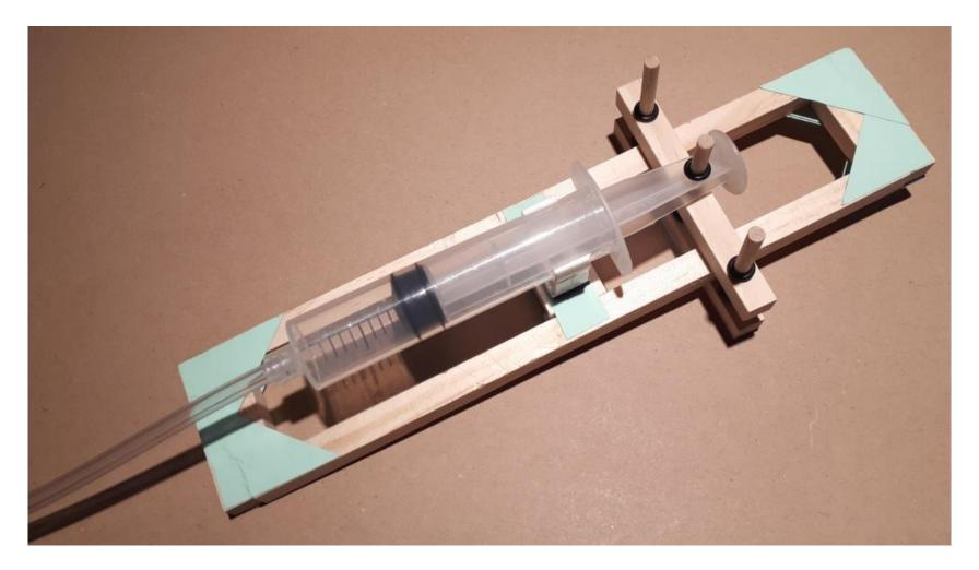
Carefully push the plunger into its barrel as far as it comfortably goes. To operate the clamp attach the other syringe, fully open with its plunger out, onto the tubing and then press its plunger in. The clamp will close. Pull the plunger out and the clamp will open
