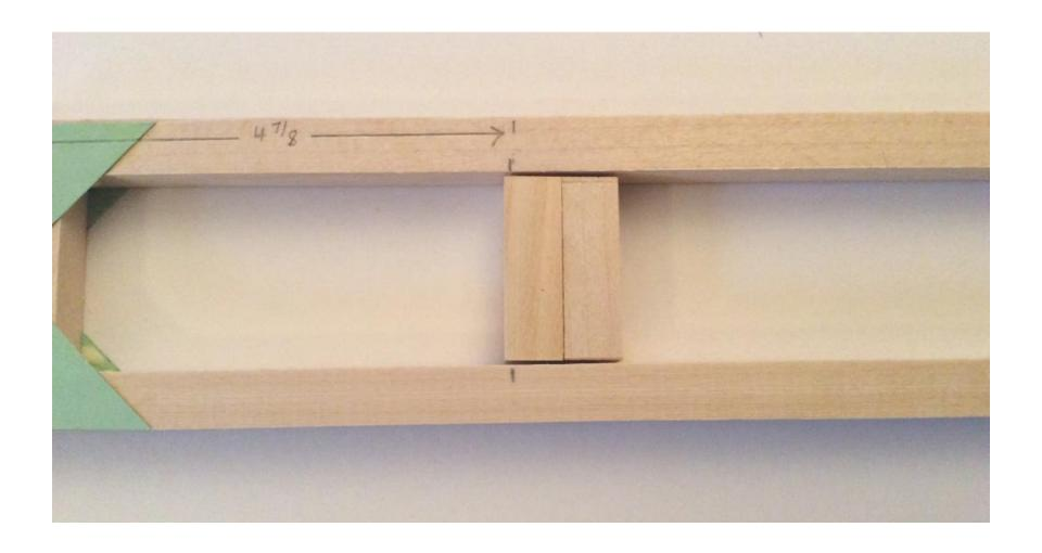
From the green gusset card cut a rectangle  $\frac{3}{4}$ " by 2" – (19mm by 51mm) and glue it to secure the two  $\frac{1}{4}$ " – 32mm pieces to the frame. Allow to dry otherwise the white syringe holder will not hold.
