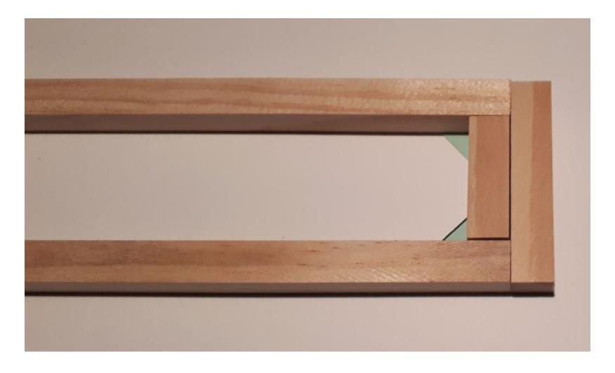
Place a  $1\frac{1}{4}$ " -32mm piece so that it lies between the long pieces of the frame  $4\frac{7}{8}$ " – 124mm from one end
