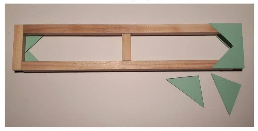
On the other side of the frame glue two  $1\frac{1}{4}$ " – 32mm pieces into the smaller ends. Secure them with glue and with four corner gussets, one on each corner.
