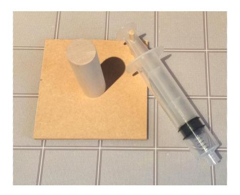
Strip off the backing from the white clip and firmly press it onto the centre of the wheel and insert this piston-syringe platform into the available hole
