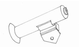
This is the standard method for connecting a piston-syringe to a base so that the piston-syringe can rotate vertically. Three small pieces are joined so that an axle will rotate in the aligned holes. Alternatively white axle holders and 3 small pieces without holes are joined, as shown.
