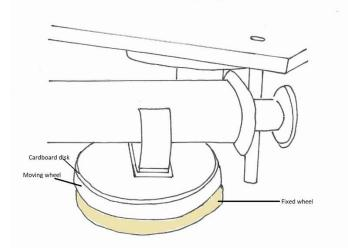
A diagram illustrating the arrangement for connecting a piston-syringe, with a hole in its plunger, to a square platform. The lower wheel is fixed. The clip is firmly pressed onto a cardboard surface.
