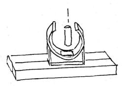
A good idea! A hole is drilled into a base formed by two strips and through the base of a white clip. A small dowel, sanded to size, is used to fix the clip to the base
