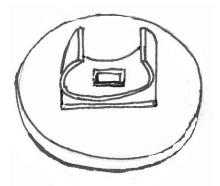
A white clip can be used instead of a gray one. The footprint of the sticky pad beneath the clip is small and therefore cardboard is used to ensure a strong connection.
