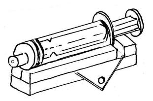
Another great idea! A way is required to stop the barrel of the piston-syringe moving forward. The base has two layers, the top layer is formed by three pieces as shown.
