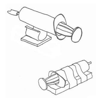
Gray and white clips are provided for attaching piston-syringes. Both have sticky pads on their base. The gray clips accommodate a 20cc syringe and have a larger footprint. The smallest of the white clips is for a 10cc syringe.
