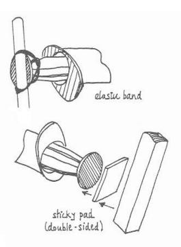
Using an elastic band and a stirrer or popsicle stick is a useful way of lining things up temporarily.
